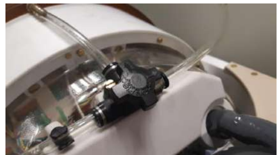
Figure A - 2: (L) Water pouch and Silicone tube with fittings, ® Air release Valve opening
