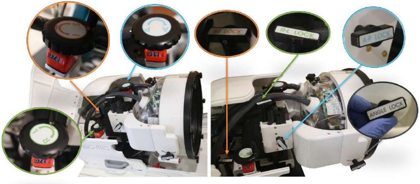
Figure 3-10: Mechanical Positioning Unit. Levers (Left), Locks (Right).
