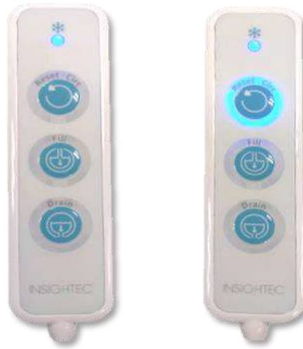
Figure 3-19: Water System Remote Controller States: Idle (Left) and While Circulation Is Active (Right)
