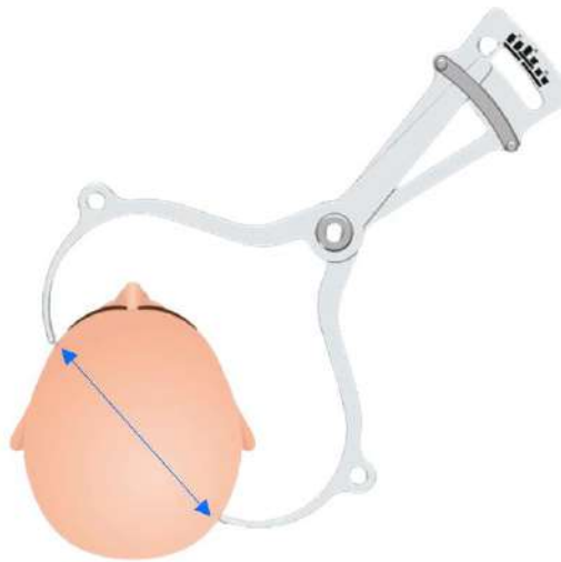
Figure 1-13: Exablate Caliper for Head diagonal measurement and combination estimation
