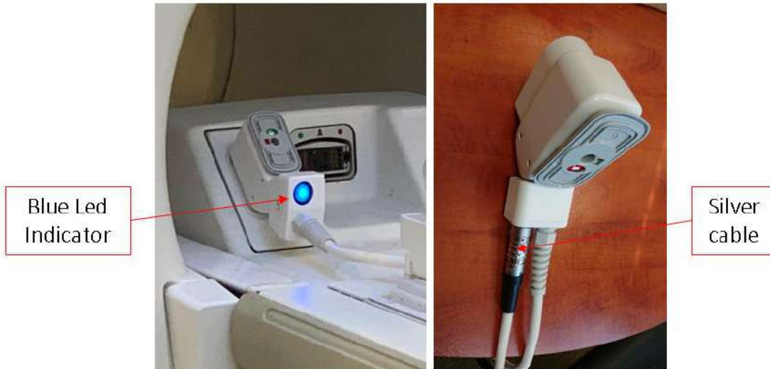
Figure 1-23: Examples of MR connectors
