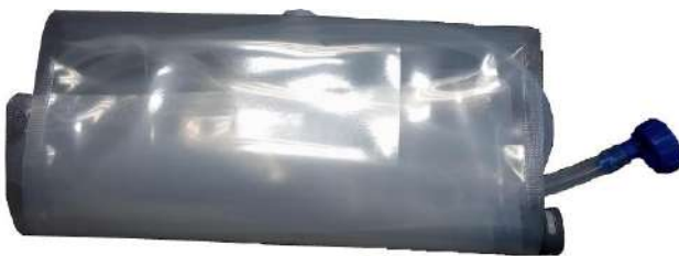
Figure A - 2: (L) Water pouch and Silicone tube with fittings, ® Air release Valve opening
