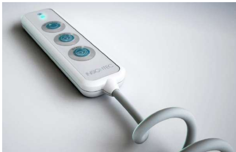
Figure 3-18: Water System Remote Controller
