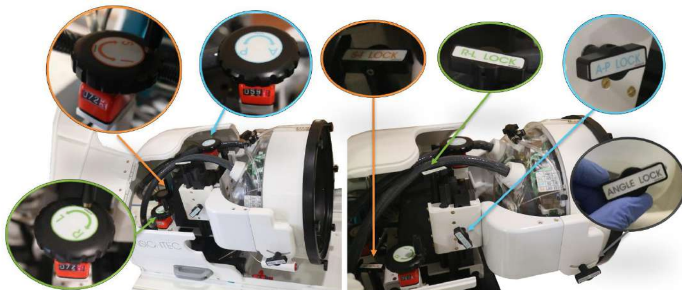
Figure 3-10: Mechanical Positioning Unit. Levers (Left), Locks (Right).
