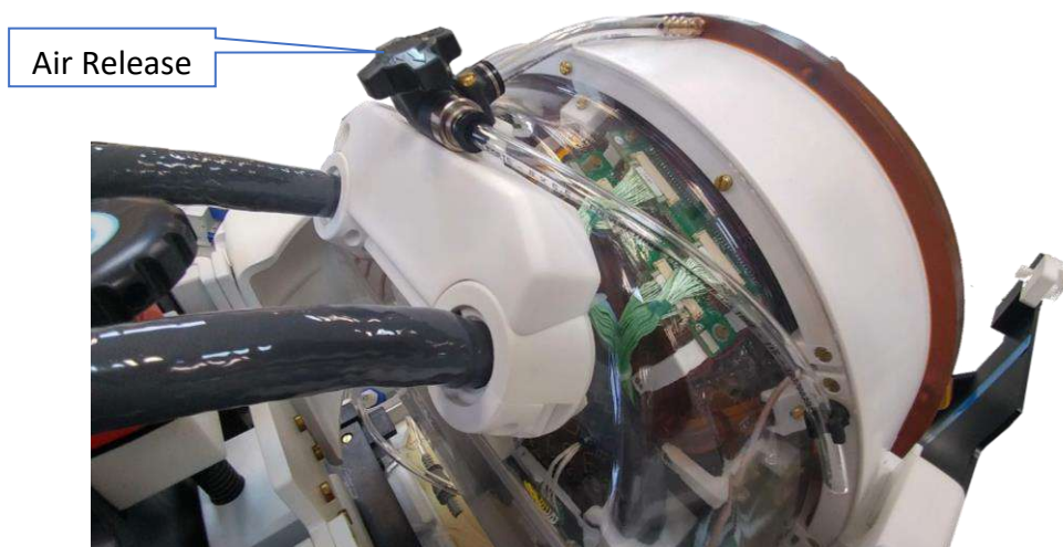
Figure 12-11: Air Release Valve (open)
