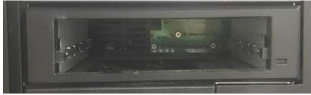
Figure C-5: PCs Hard Drive Bay when dirsk is removed
