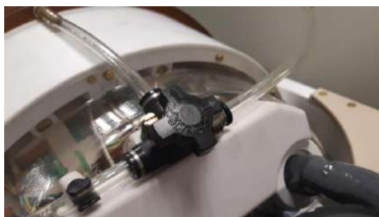
Figure B - 2: (L) Water pouch and Silicone tube with fittings, (R) Air release Valve opening
