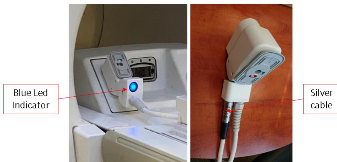
Figure 1-23: Examples of MR connectors
