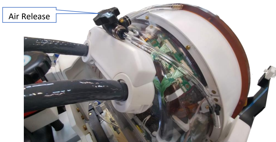
Figure 12-11: Air Release Valve (open)
