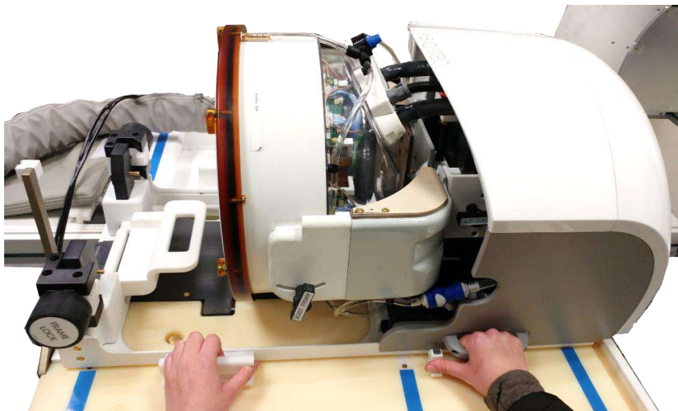
Figure 3-6: Transferring the HS to the MR Table
