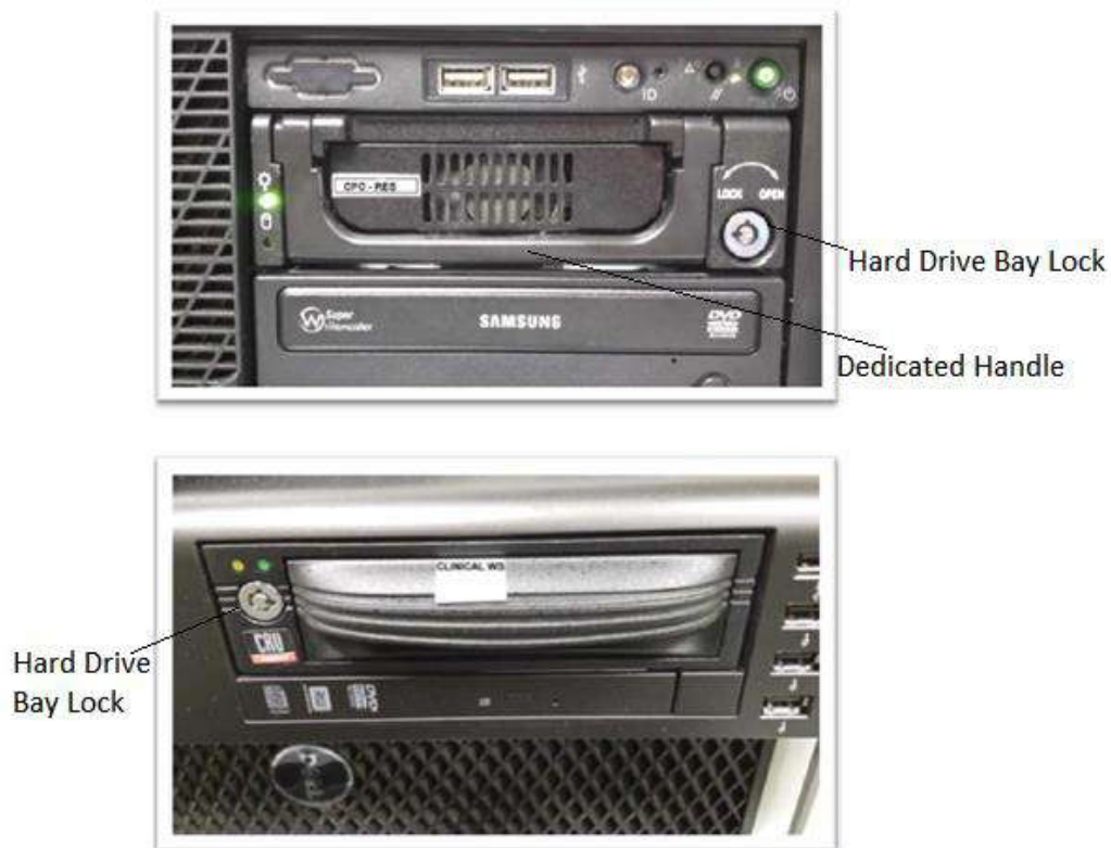
Figure D - 2: PCs Hard Drive Bay (Note Keyhole with Open/Lock Position Designations)
