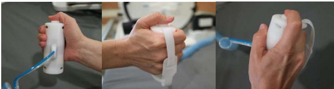
Figure 1-9: Patient Stop Sonication Button (Type 1.1)
