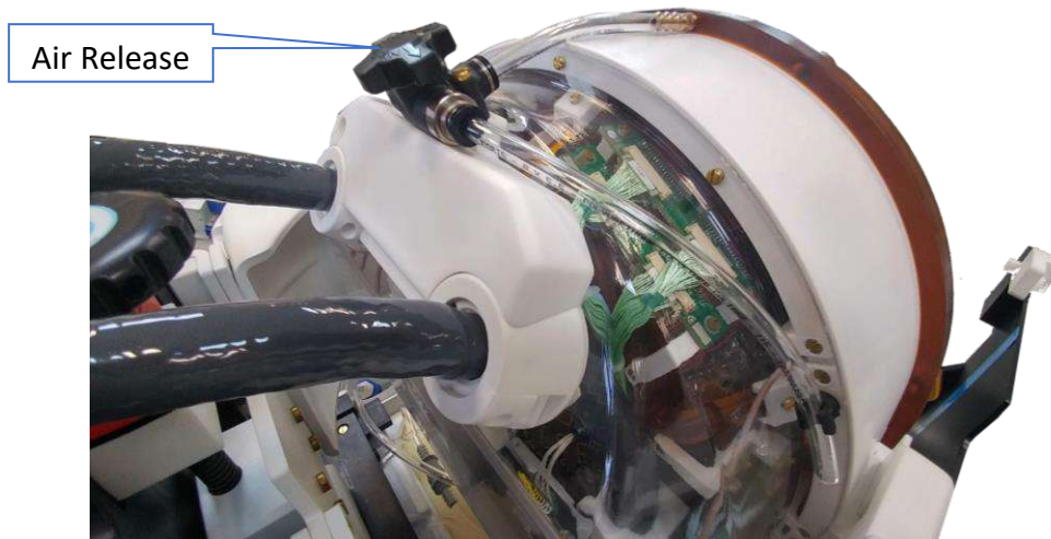
Figure 12-31: Air Release Valve (open)
