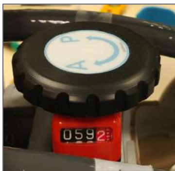
Figure 3-14: Type 1.1 A-P Positioner Lever
