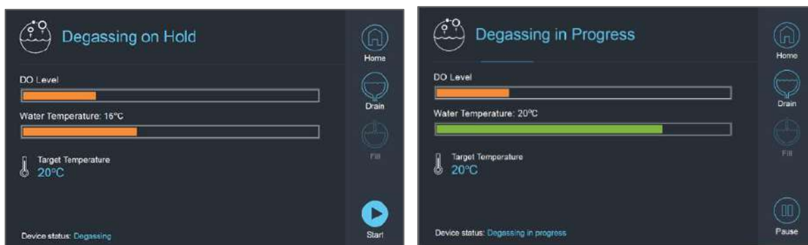
Figure 3-19: Type 1.1 Degas Mode Screens
