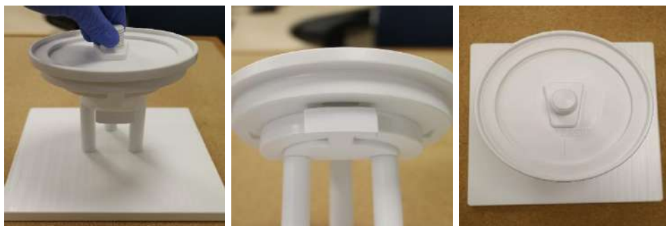
Figure 5-3: DQA Holder and Mounting Jig Assembly
