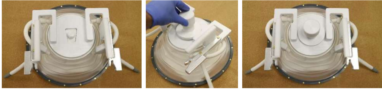
Figure 5-5: DQA Set Up Holder Assembly
