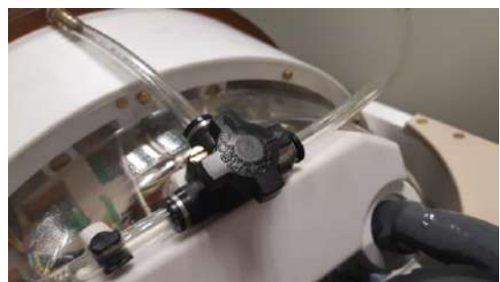
Figure C - 2: (L) Water pouch and Silicone tube with fittings, (R) Air release Valve opening
