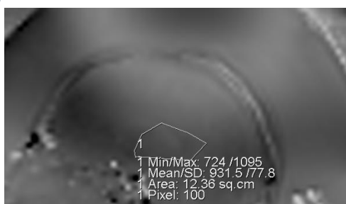
Fig. 3: ROI drawing around center of DQA Phantom
