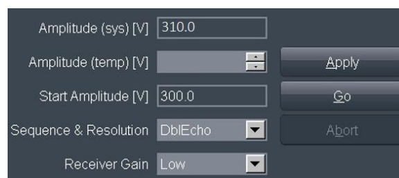
Fig. 2: Updating the Amplitude value (example, SIEMENS VE11e\VE11c)
